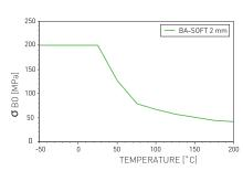
**P-T diagrams** indicate the maximum permissible combination of internal pressure and servicetemperature which can be simultaneously applied for a given gasket according its material type, thickness, size and tightness class. Given the wide variety of gasket applications and service conditions, these values should only be regarded as guidance for the proper gasket assembly. In general, thinner gaskets exhibit better P-T properties.
